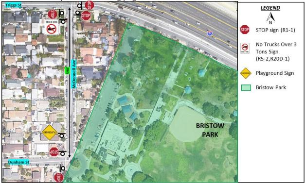
Staff reviewed the segment of McDonnell Avenue between Triggs Street and Dunham Street based on the City's Speed Hump Policy. It is recommended that speed cushions be installed along the segment specified. These traffic calming measures will aid in the reduction of both speed and traffic. Placement of official traffic control devices on public streets is guided by the California Manual of Uniform Traffic Control Devices (CA-MUTCD) Section 2B.04 for right of way assignment.
