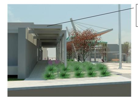
Option: omit roof over walkway on existing metal frame Savings = \$50,000
